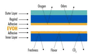
At Silgan Plastics, instead of making an entire package out of EVOH, we keep costs down by coextruding EVOH as a discrete layer in multilayer structures. This application is an ideal substitute for fluorination, which can add costs and delay speed to market.
